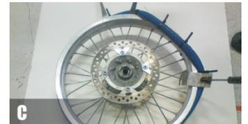
**Step 5:** Lay down the wheel (on a tire stand if possible) Start to press one of the tire sides over the rim edge. Be careful with the tire levers so you not will damage the T-Lock's sealing lips. Turn the wheel around and start to assemble the other side. Before you complete the assembly of the tire, turn the wheel upright and fill it with T-Lock Seal, 200 ml (See picture F).
