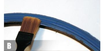
**Step 4:** Place the MX tire at the floor, apply some T-Lock Seal at the inside of the tire and the tire edge with a brush. (See picture D).
